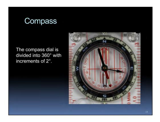
Your compass dial uses the system I have just showed you. Because of the thickness of the marks, only the even-numbered directions are shown. At the very top there is a clear arrow point lined up with 0 degrees. We call that the index mark. There is a similar mark on the opposite side at 180 degrees. If you turn the dial so that 54 degrees is at the index mark, you can read off 234 degrees at the opposite mark.
