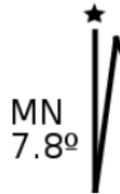
Figure 13: Magnetic declination diagram on Mount Vernon map. The line with the star stands for true north; the half arrow stands for magnetic north.
