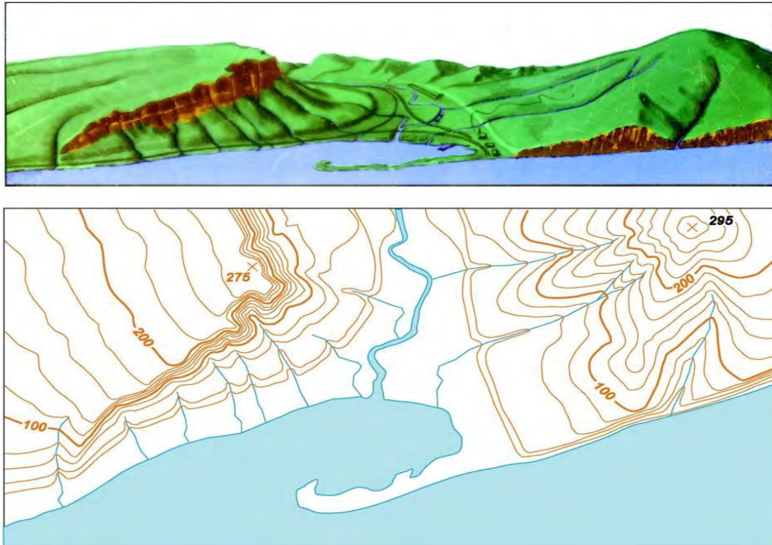
Figure 4: Perspective drawing of a landscape and contour map of the same landscape. Contour interval is 20 feet.
