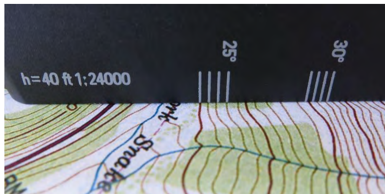
Figure 3 Measuring the slope of an area with scales on the MC-2 compass. The lower part of this avalanche chute has a slope of 25°.
